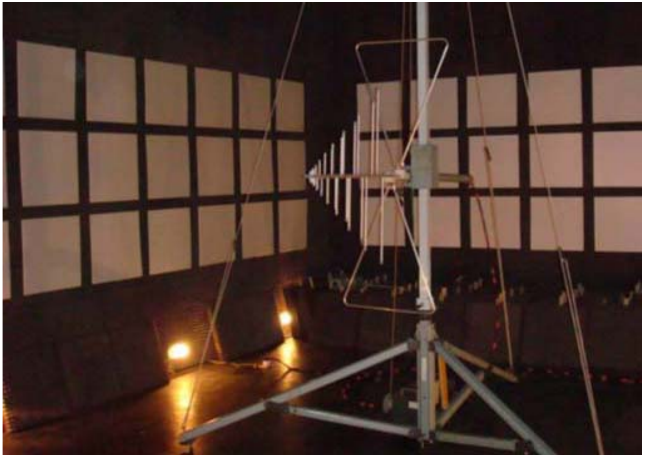
Fig 5. Semianechoic chamber with remote controlled turntable
