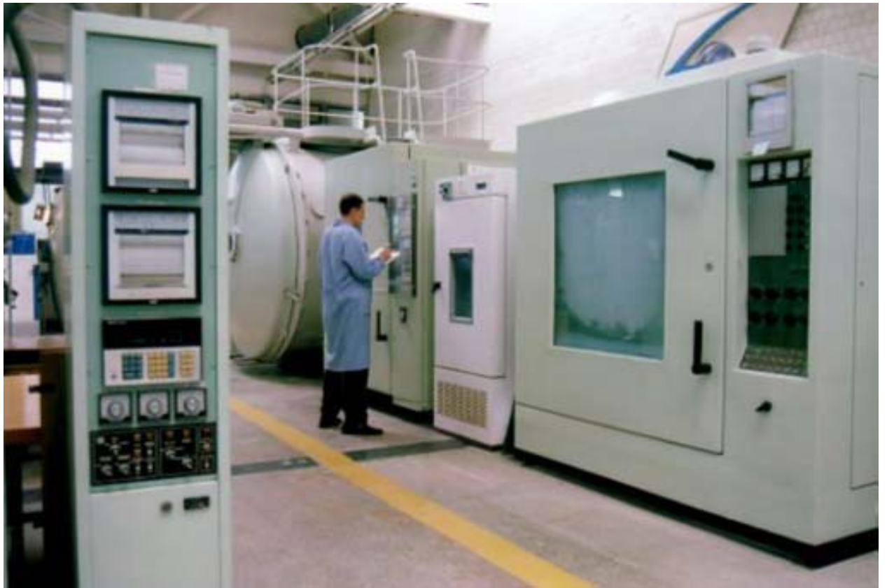
Fig.3 Site for climatic testing of the large dimensional samples of marine radio equipment
